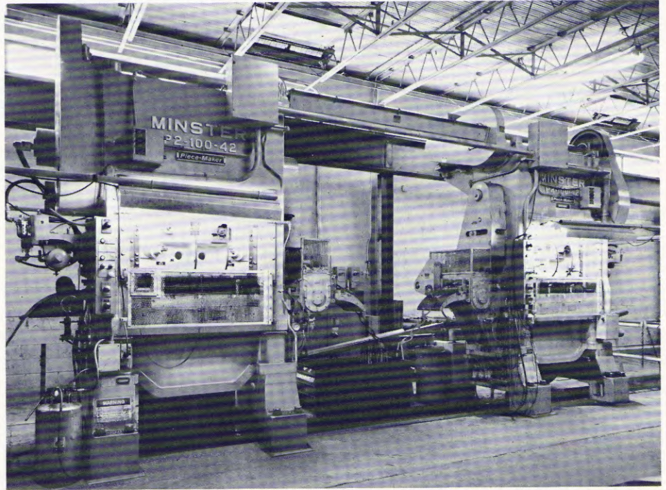
Tandem P2-100 lamination presses run in synchronization producing stator-rotor sets from scroll cut strip steel.
