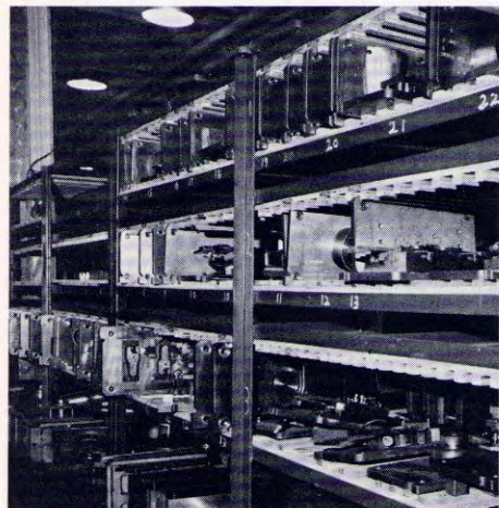
Simplified Die-Namic dies reduced die storage requirements by 50%.
