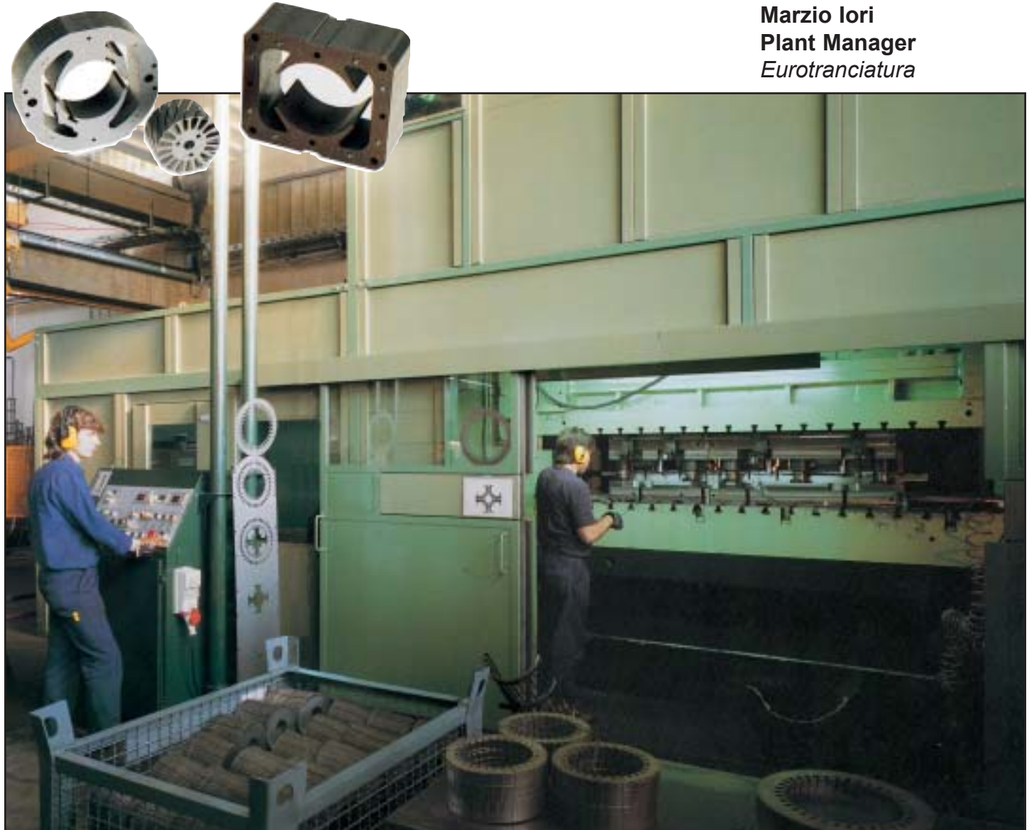
Utilizing larger presses, Eurotranciatura is able to blank laminations with an outside diameter of up to 600 mm.
