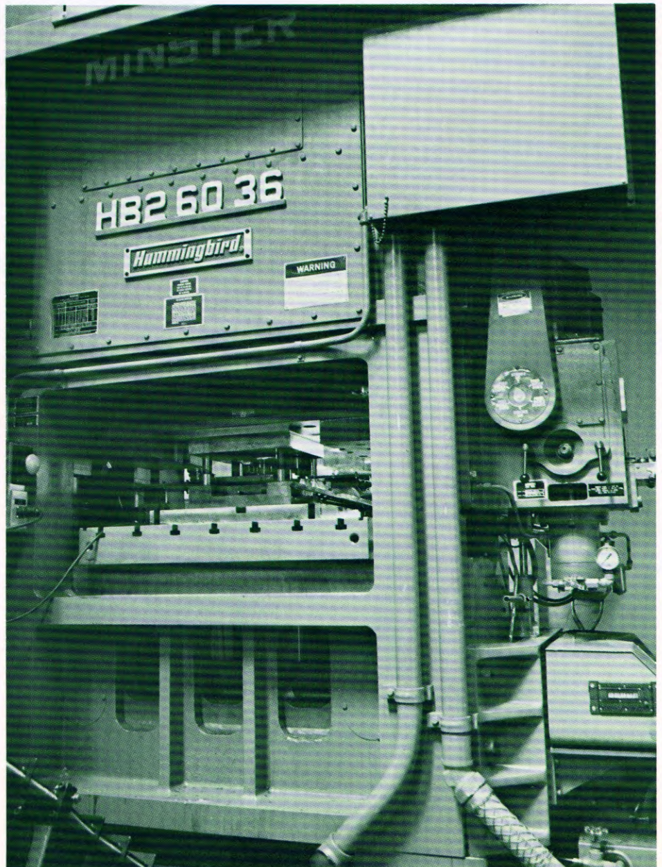
With enclosure doors open the slide, die area and Minster high speed roller cam feed can be seen. Note part chute coming out from under press bed.
