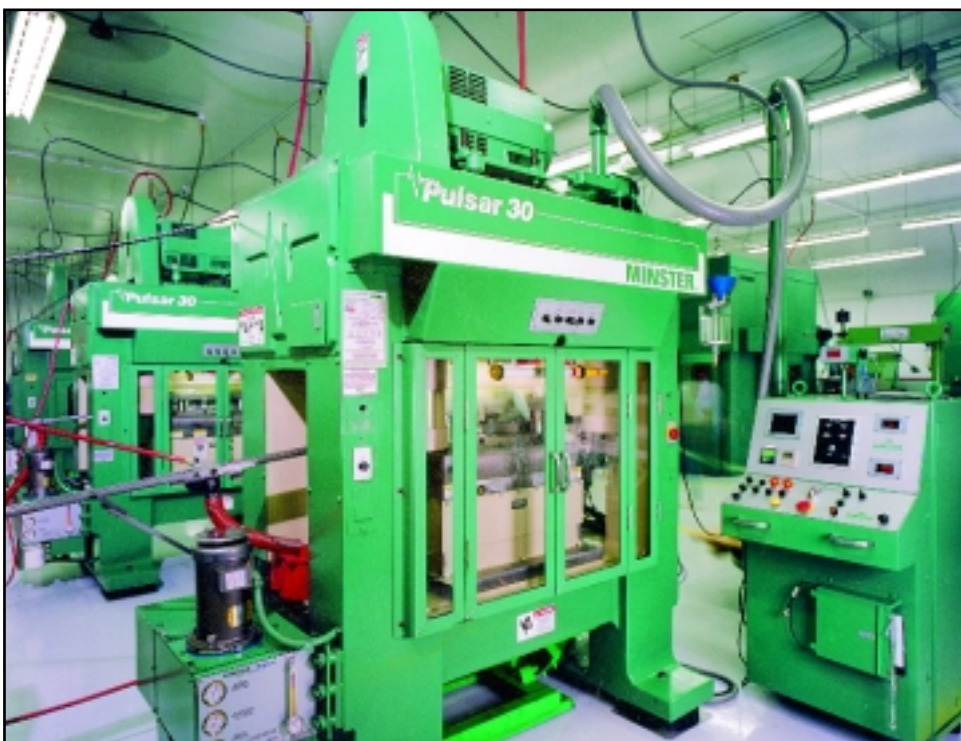
Minster Pulsar 30 ton presses are handling some of the high volume stamping jobs at Midwest Tool and Die.
