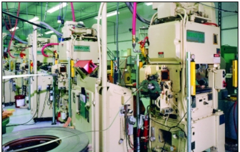
Minster TR2-15 presses handle some of the lighter high speed jobs at Midwest Tool and Die.
