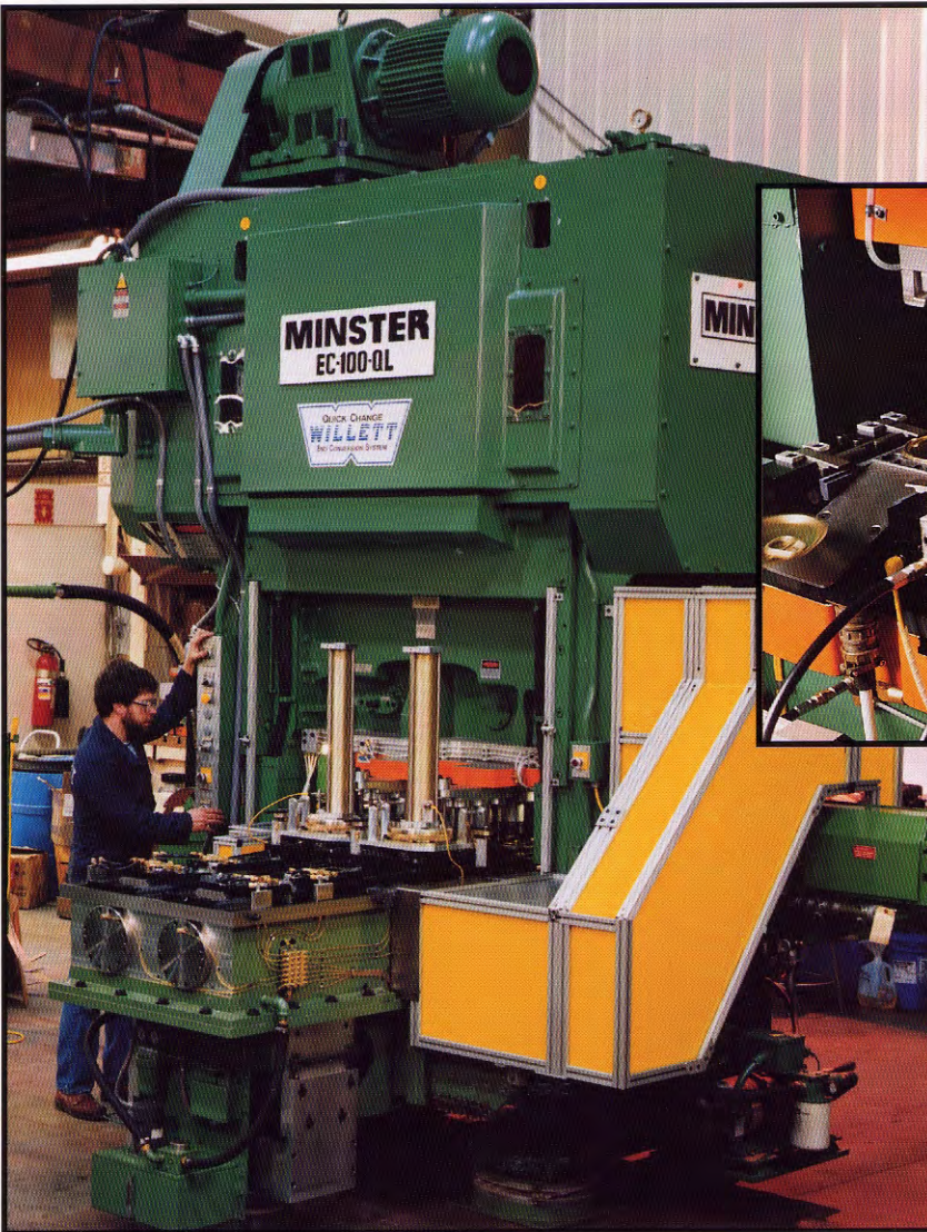
A Minster EC-100-QL Press and Willett Tooling produce food container lids in a system headed for France.
