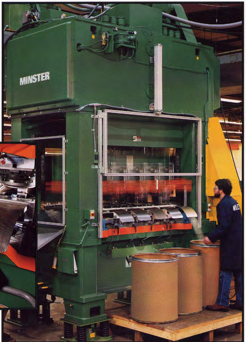
A Minster SAS-H100-72 Press and Willett Tooling produce the bottoms of cookie tins in a system headed for Denmark.
