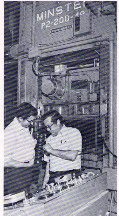
Cecil Combs, Foreman left, and Bruno Marchi, Plant Manager inspect progressive die strip being run in a Minster Piece-Maker press.
