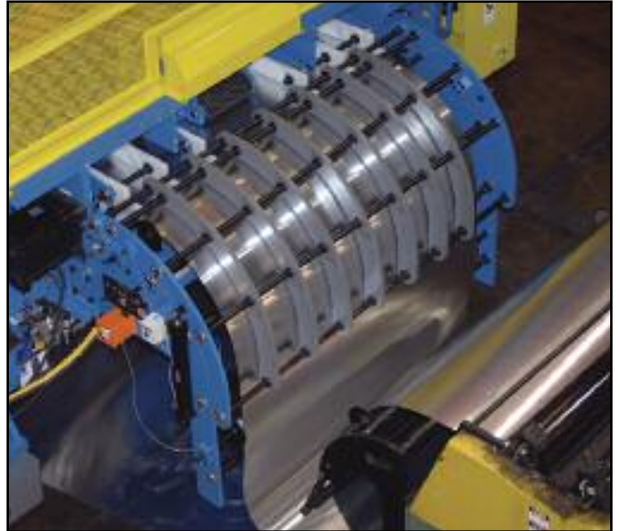
The Minster Container Servo Feed provides accurate feeding for Minster Shell and Cupping Presses; and the optional Swing-Away feature allows easy access to the die and tooling.
