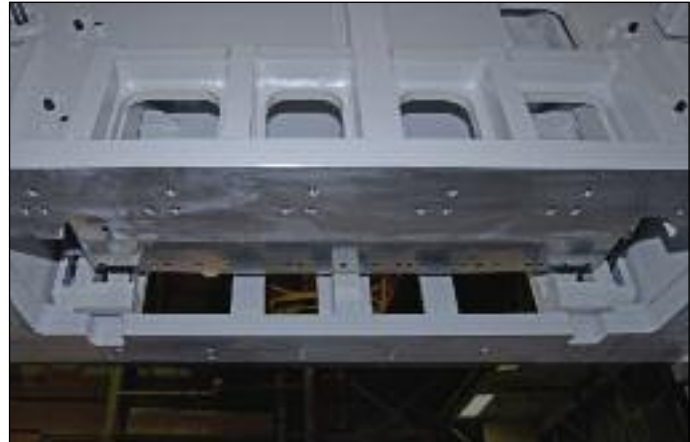
View looking up at slide faces. Outer slide guided within the uprights, inner slide guided within the outer slide.
