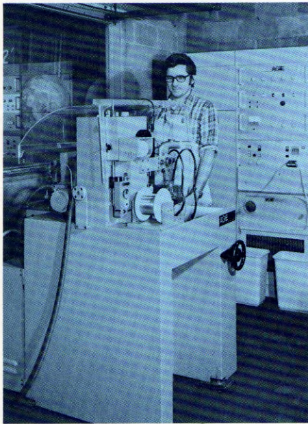
Example of Stan Karr's belief in the value of buying quality equipment is this tape-controlled AGIE "Traveling Wire" EDM machine. One of 50 in the U.S.A., it is used to cut intricate die components from steel or carbide to \pm .0002 " tolerance in the tool-making department.
