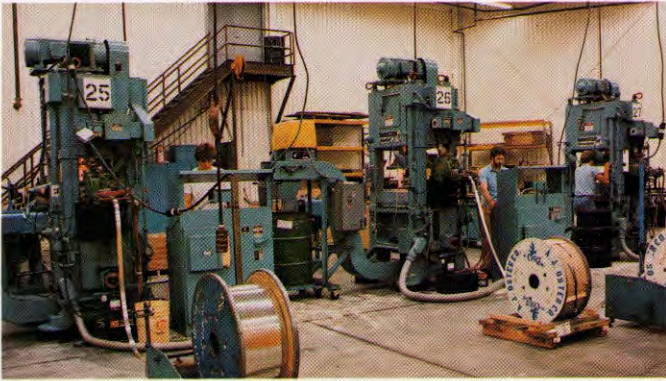
These Minster Hummingbirds were Interlock's first stage in their program to increase press productivity.
