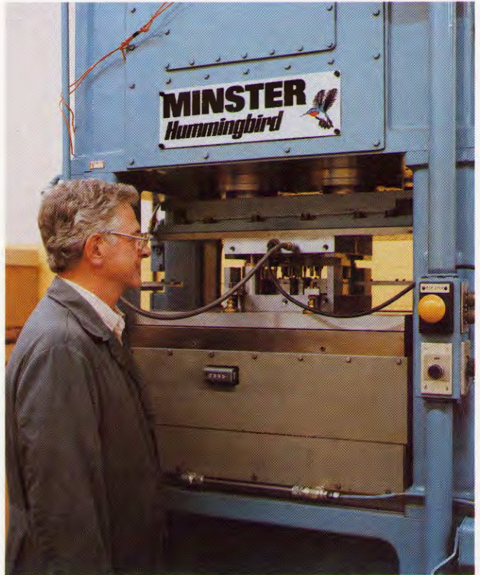
A Minster Hummingbird is used at Interlock Technical Center for die tryouts.
