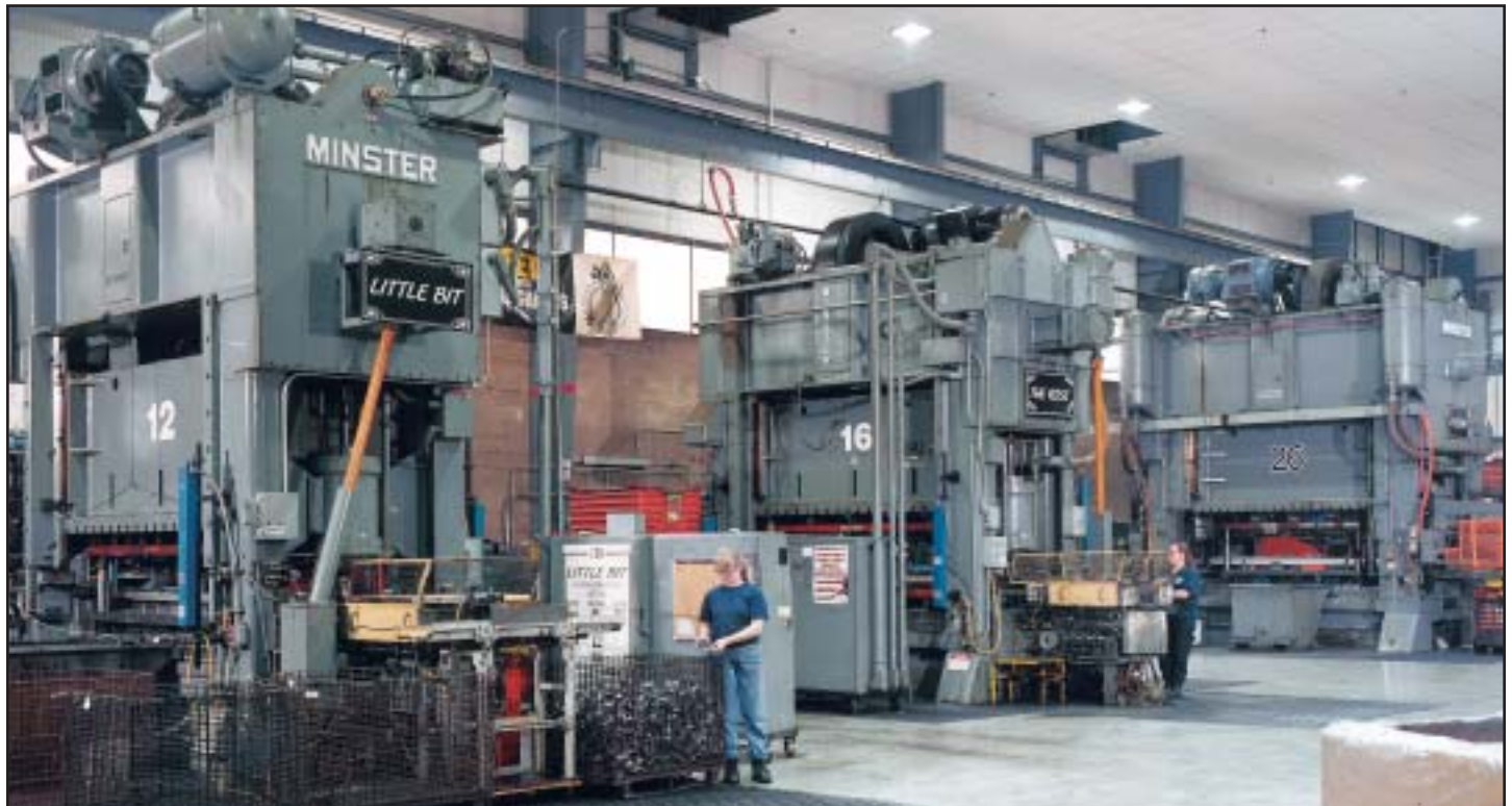
Minster presses are used for several transfer applications at Bayloff Machine and Die Co.
