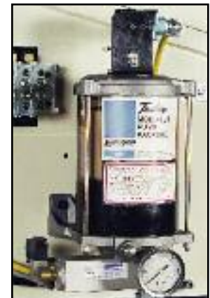
Automatic Lube System
