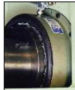
Large Surface Area Drag Brake
