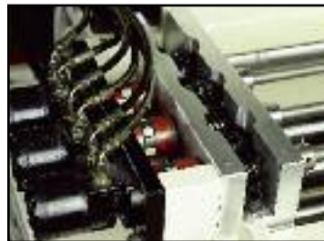
Independently-Adjustable Work Rolls
