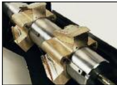
Wedge-Type Mandrel Expansion
