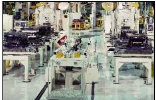
Pre-Staging With Auxiliary Storage Racks
