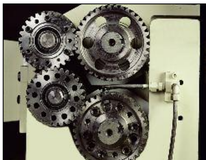
Helical Gearset Designed With Zero Backlash
