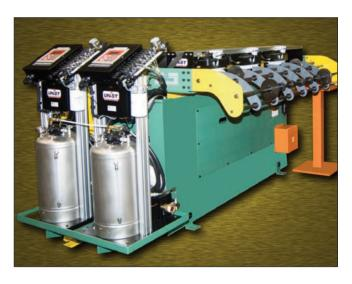
**NOTE:** Depending on customer preference, Unist lubricating units can be integrated into the feed or catenary.
