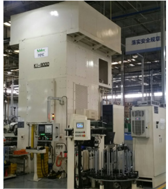
800 Ton Knuckle Joint Press with Automation System for Powder Forming Application
