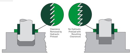
P2H Adjustment Screw with Hydraulic Lockup
