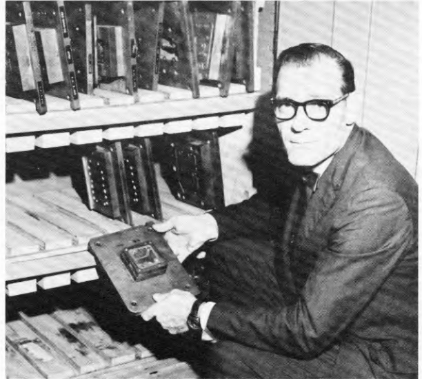
Mr. Cecil Lenhart, Manufacturing Engineer, shows one of over twenty compound dies used with the Minster Die-Namic press. Dies are stored in a closed metal cabinet within a few feet of the press. Plate-mounted dies are filed in easily accessible, vertical position requiring very little space.
