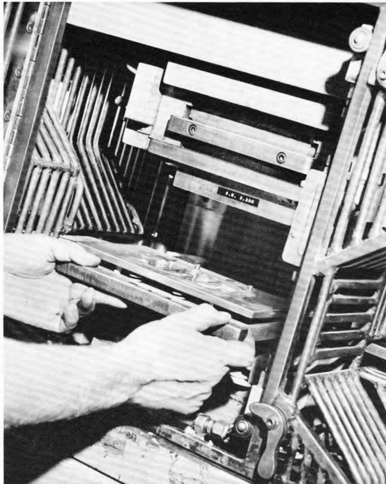
Unique design guard with plexiglas door.
